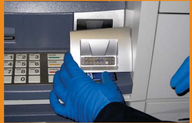
ATM skimmers attach to an ATM over the card reader and often copy your card information and PIN.
